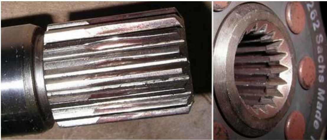
R1150GS Spline wear at 75k km. Clutch hub splines very worn, input shaft with noticeable wear
