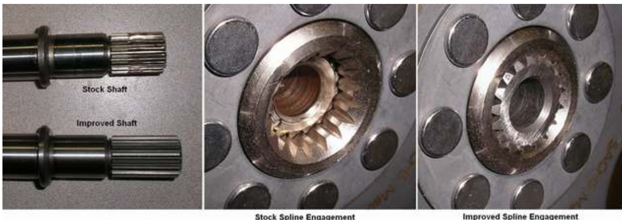
R1150GS Spline wear at 75k km. Clutch hub splines very worn, input shaft with noticeable wear
